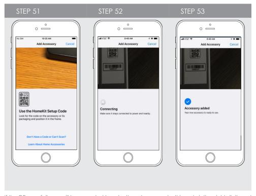
If the QR scan fails you will be prompted to enter the setup up code, this code is the eight-digit number located in the top right of the QR code.
