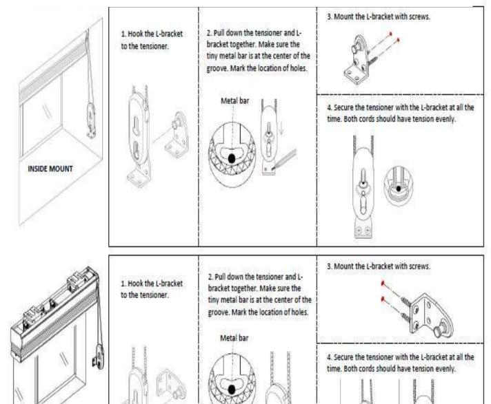
The tensioner and L-bracket must installed properly before operating the clutch shade.
