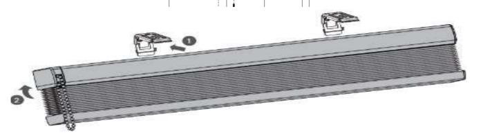
IMPORTANT-THE CLUTCH CELLULAR SHADE WILL NOT OPERATE WITHOUT THE SAFETY TENSIONER PROPERLY INSTALLED. FOR SAFETY REASONS, THE CORDLOOP MUST BE SECURED TO ENSURE IT IS UNDER TENSION AT ALL TIMES.
