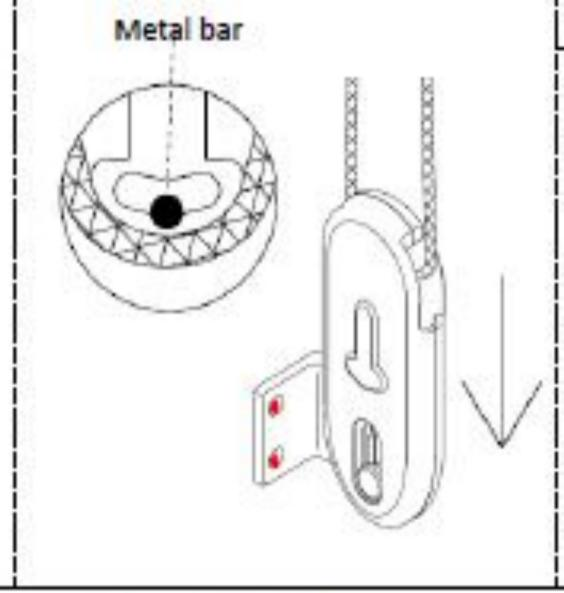
3. Mount the L-bracket with screws.
