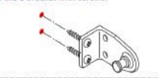
4. Secure the tensioner with the L-bracket at all the time. Both cords should have tension evenly.
