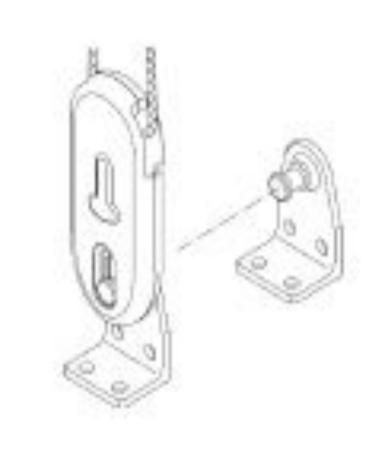
Pull down the tensioner and Lbracket together. Make sure the tiny metal bar is at the center of the groove. Mark the location of holes.
