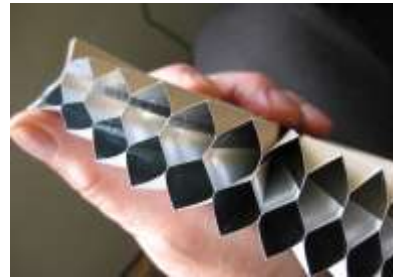
cellular material - one cavity has both sides aluminized mylar, the other has one side aluminized mylar
