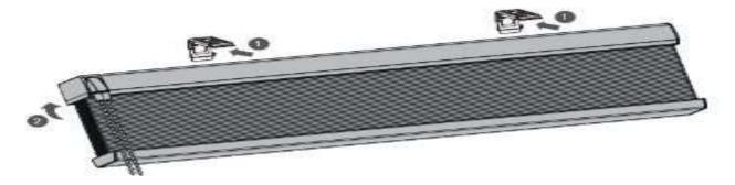
**Installing your wands**: Each wand snaps into the pull connector located next to the headrail by pressing the ball into the connector and then moving the wand so that it is perpendicular to the shade.
